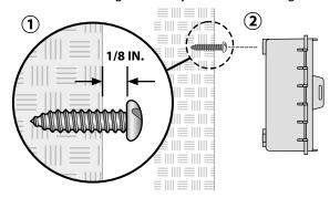
3 Open the front panel, and drive three additional screws through the open holes inside the controller and into the wall, as shown.
