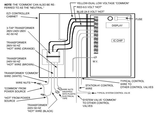
**NOTE:** BE SURE TO USE A WIRE NUT AND PROPERLY TAPE EACH OF THE REMAINING "HOT" WIRES FROM THE TRANSFORMER (TWO WIRES) TO COMPLETELY ISOLATE THEM AND PREVENT "SHORTING OUT."
