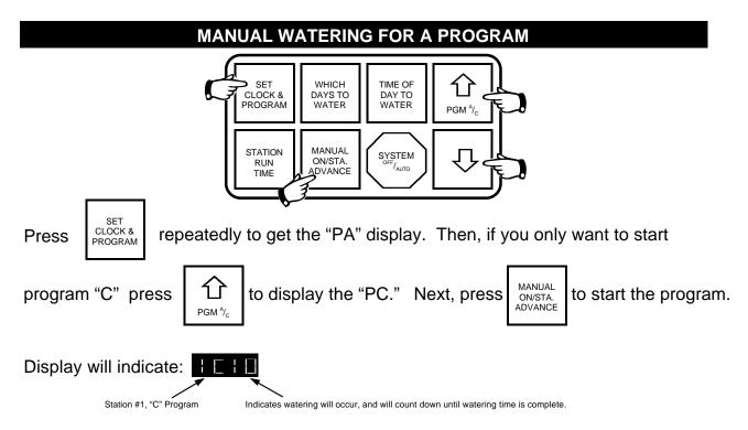
Note: When a station is watering, the station number and program will appear as the first two digits in the display. The digit(s) to the right will blink throughout the watering time. The manually started program will water all stations on that program and then return to automatic mode and await the next scheduled automatic start.
