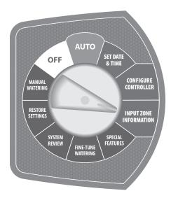
1 The INPUT ZONE INFORMATION screen will appear with the **Zone**Setup Wizard blinking; press the SELECT button.
